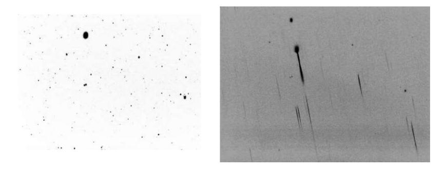
Slit less spectrograph produces elongated images of point-like objects. If we achieve point-like meteor images of meteors with our adapter, we surely shall be able to have spectra of meteors about 7<sup>m</sup>...8<sup>m</sup>
