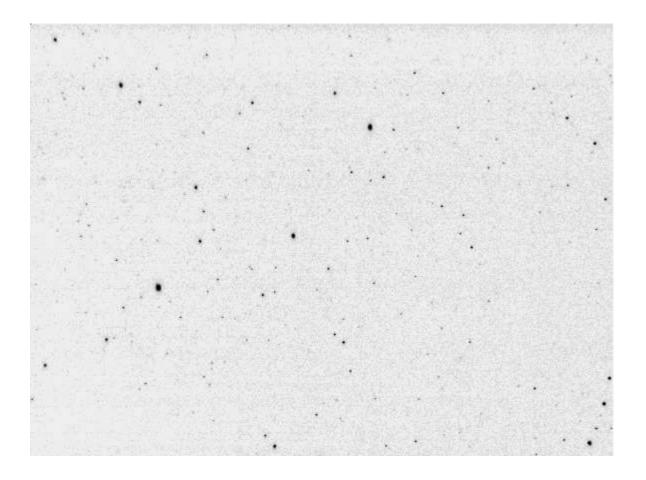
A camshot by TV camera on the base of matrix ICX285 with high speed lens Canon EF 85 mm f/1.2 at 1 sec exposition
