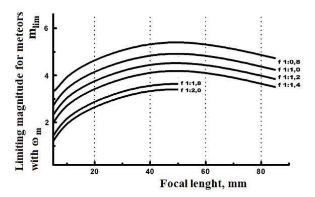
The limiting magnitude for meteors dependence on lens parameters for well-known WATEC 902 LCL 902 or its successors, when angular meteor velocity  $\omega_m = 5^{\circ}/\text{sec}$
